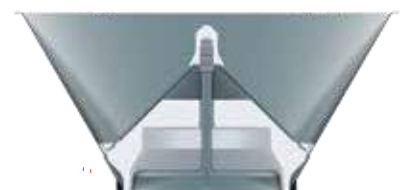
Cross-section showing the position of Cone Valve in an IBC
